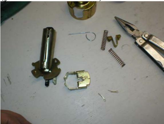
Parts released when removing inside spindle
