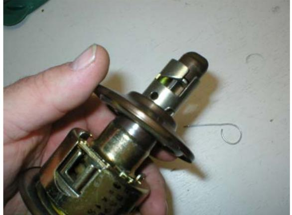
Remove Rose (remove screws to take off mounting plate {not shown})
