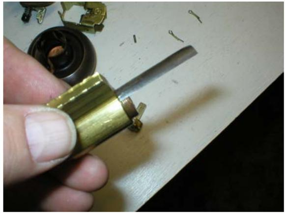
Shim the lock open (you would not have done this if you could have picked it, in the first place). Service, Re-pin or make a key for the lock.
