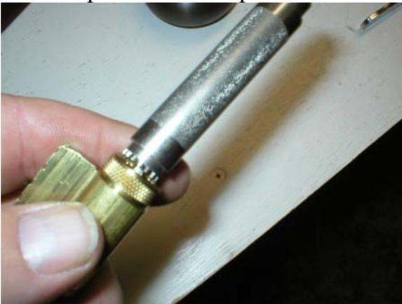
Now you can use your Schalgé cylinder nut tool to remove the Nut.
