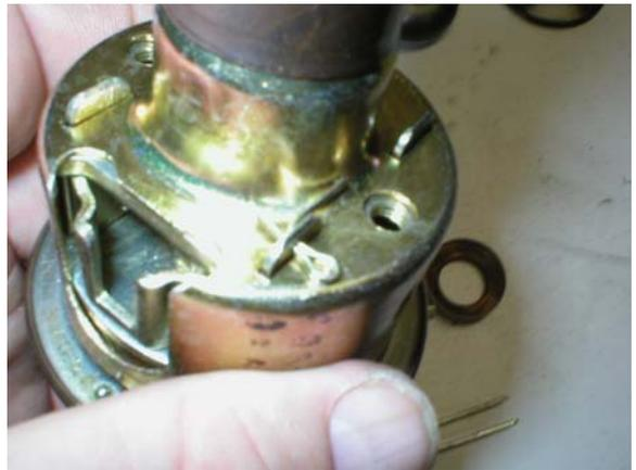
Install cotter pins test operation of spindles (inside and out)
