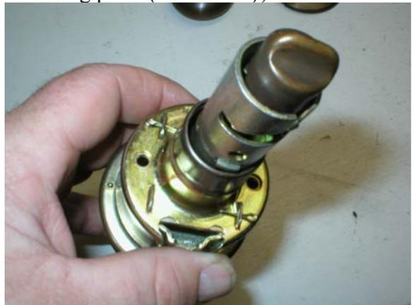
Knob ready for disassembly (note cotter pin)
