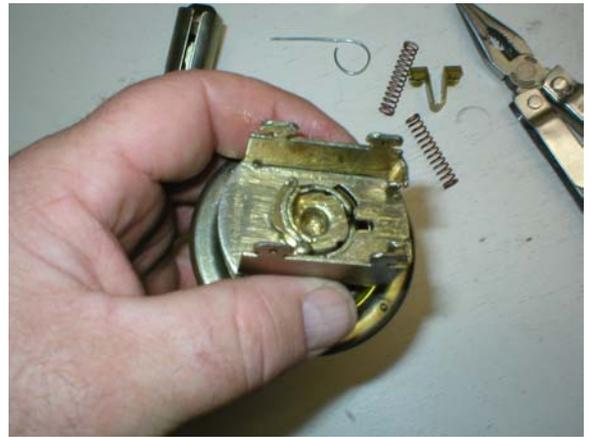
Tip up the exterior knob spring cage so you can see the inter-workings. Note the slot for the locking shaft and the dimple in the locking cam (this is spring loaded to allow the locking shaft to spring back to the unlocked position)
