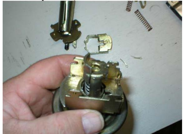
Pull up on the locking cam notice the spring. At this point on some locks you can depress the knob retainer and it will "slip" by depending on many factors: age, wear, style or type of cylinder tailpiece.
