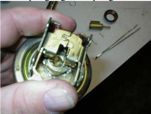
Depress and hold spring cage to insert lock shaft and interior side spindle
