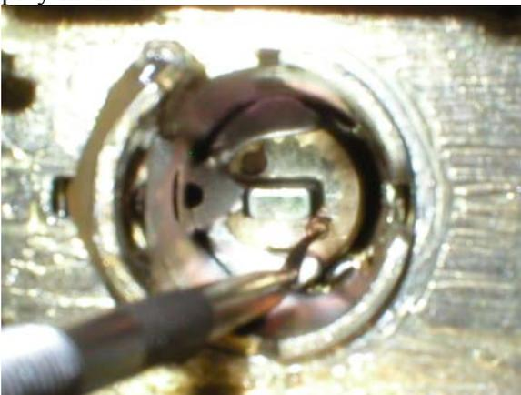
Another view of probe on nut retainer to show location (on some levers they use a larger knob retainer that will not allow this method of cylinder removal, also if someone put a washer in behind the cylinder you may not be able to access this retaining pin)
