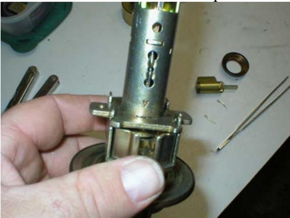
Insert lock shaft into dimple and the lock slot, interior side plate sometimes will get out of alignment. USE a LOT of Patience.
