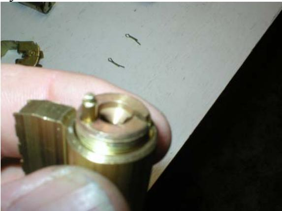
Nut removed notice the retaining pin remove pin and spring (so you don't lose them)
