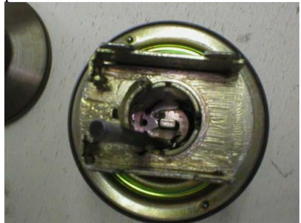
When you have enough space, use a pair of tweezers to pull up on the tailpiece, depress retainer far enough to allow the tailpiece to turn.
