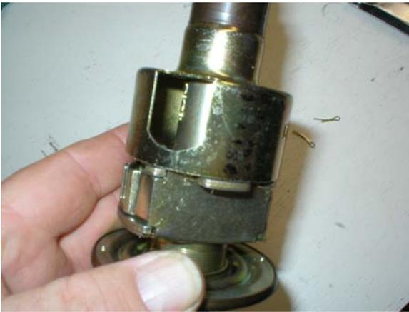
Depress latch retractor and slide sleeve off, sometimes you have to turn to get it to slide off.
