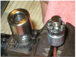
Outer shell removed, notice the numbering on the face of the shell
