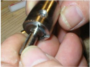
Remove the retaining pin (this is hardened steel)
