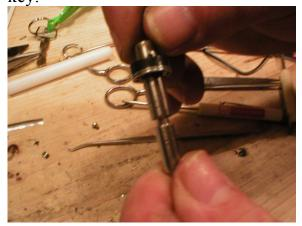
Center shaft and upper-sleeve; notice the spline cut in the shaft. Service the lock (Rekey or reset to the original key).
