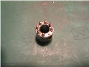
Top pins and spring case notice "7" pins this is an "8" pin lock there is 1 "dead-pin" that rotates as the lock is changed with the Change-a-Matic key.
