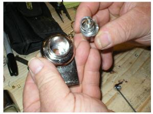
Remove the cylinder from the case there is a heavy spring (helps to pop out the cylinder when it is unlocked)
