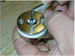
Next remove the Allen screw from the tailpiece crossbar and remove the crossbar notice the grooves on both sides of the tailpiece.
