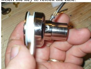
To service the lock remove the screw on the side, this screw keeps the tailpiece aligned and retains the cylinder in the casing.
