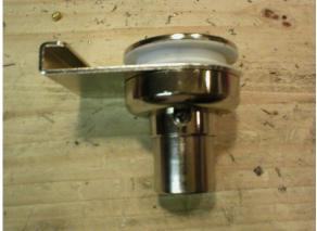
This lock pushes in and turns to lock it is a key retaining lock (that is where most of the trouble begins, the clerks have a big key-ring full of keys and they leave it hanging in the door while serving a customer) The tab on the outside of the lock gets a little worn and then can be pried out of the lock with little effort, then they cannot insert the key to relock the case.
